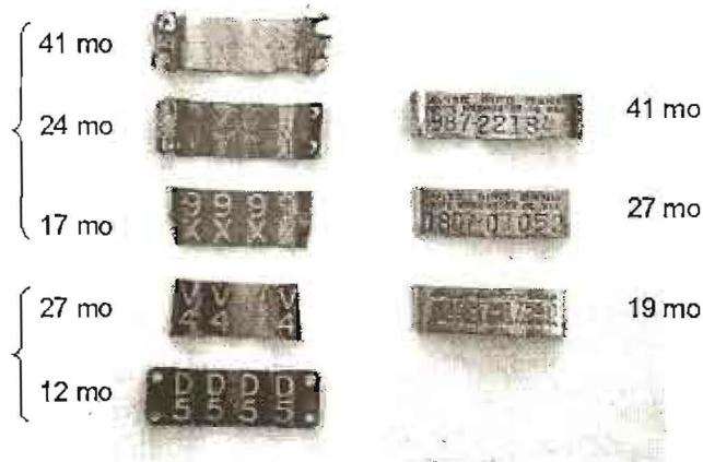
**Fig. 1.** Aluminum color anodized (left) and aluminum USGS (right) bands recovered from Common Ravens (*Corvus corax*) in NW Wyoming. Two different manufacturing batches of color anodizing (a and b) were used to determine if the anodizing process was compromised and increased the rate of band wear. Both types of bands exhibited erosion on the margins, but surface wear was much more pronounced on the color bands.
