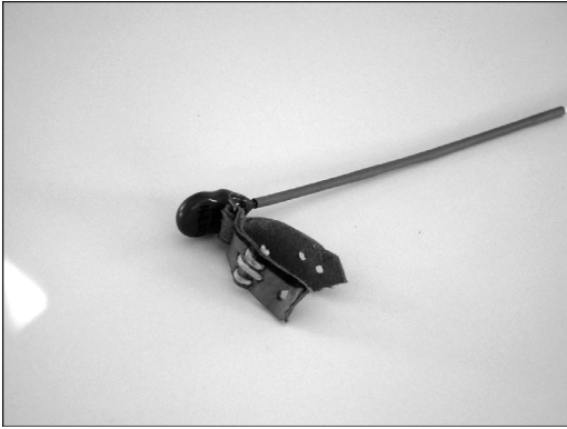
FIGURE 3. Tarsal mount transmitter used on fledgling Common Ravens. Transmitters were equipped with 2-mm cotton stitching as a break-away feature and colored shrink tubing on the antenna for ease of identification.
