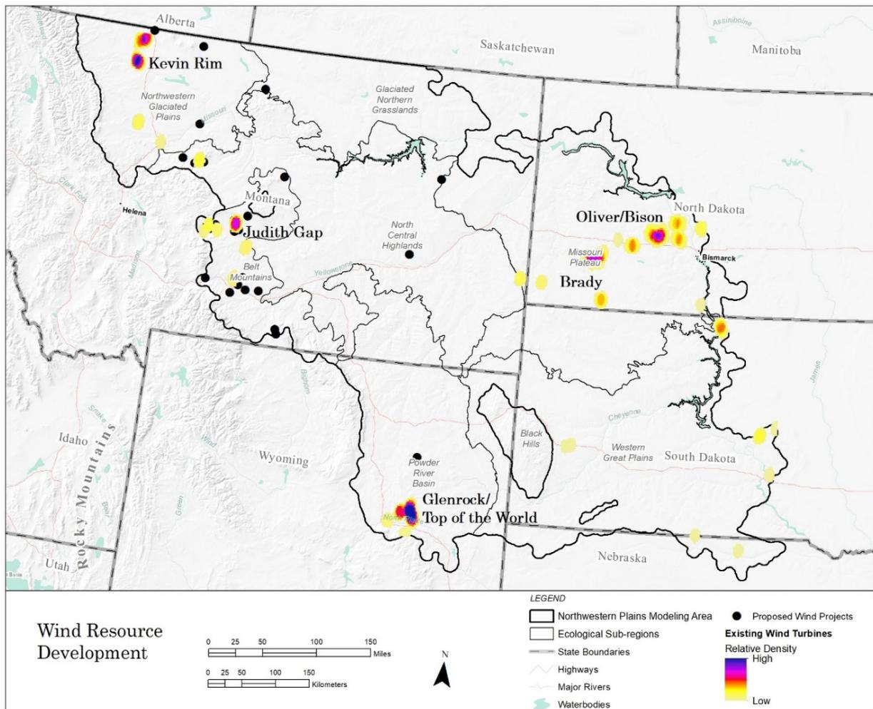
**Figure 3.4.** Density of industrial wind energy turbines and proposed wind projects in the Northwestern Plains golden eagle conservation assessment area. Common names of wind facilities are presented for reference but may not reflect all operators or facilities within each area.
